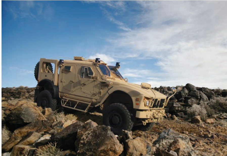
The Oshkosh M-ATV supports the addition of armour upgrades such as Underbody Improvement Kits (UIK). The advanced M-ATV design uses Oshkosh's TAK-4 independent suspension system to accept UIKs and other upgrades without impacting payload or off-road mobility
