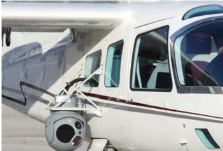
Light ISR system from Selex ES, a low-cost airborne surveillance solution
