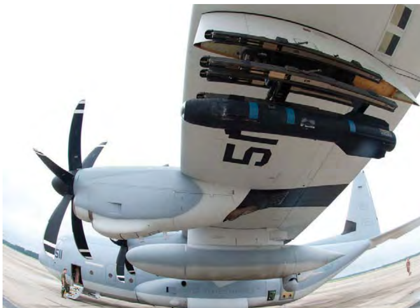
Instead of a KC-130J hose refueling pod on the outboard wing station, Harvest Hawk has an M299 quad-mount Hellfire missile launcher
