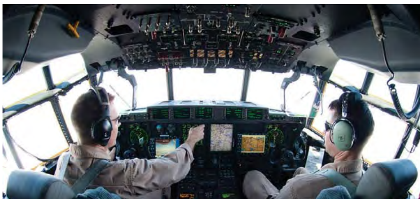
In Harvest Hawk, two additional display monitors are permanently installed on the flight deck primarily to allow the pilot to see the sensor images
