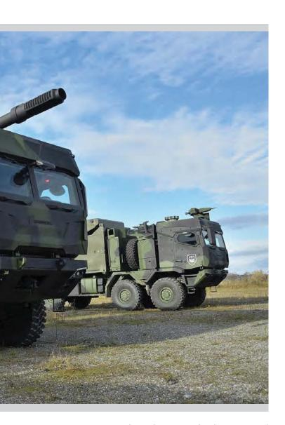
As an option, HX3 trucks can be equipped with an armoured cab, whose protection level can be modularly augmented. In addition to conventional camouflage, the new generation of vehicles feature a digital stealth mode: if necessary, all data transmission and receiver functions can be switched off to
