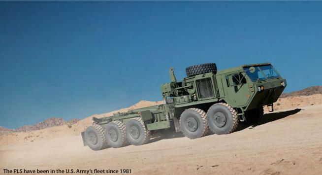
power, maintenance and safety to the battlefield. Its 500 horsepower Caterpillar C15 engine offers greater horsepower than its predecessor, so it can traverse challenging environments easily and efficiently.
