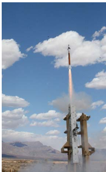
EAPS successfully conducted the first guided flight test to characterize the seeker, guidance, navigation and control systems of its MHTK Interceptor
