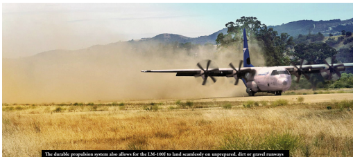
The durable propulsion system also allows for the LM-100 to land seamlessly on unprepared, dirt or gravel runways
