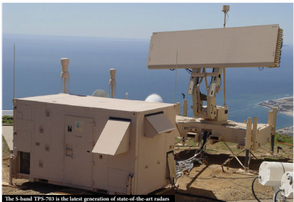
The S-band TPS-703 is the latest generation of state-of-the-art radars
