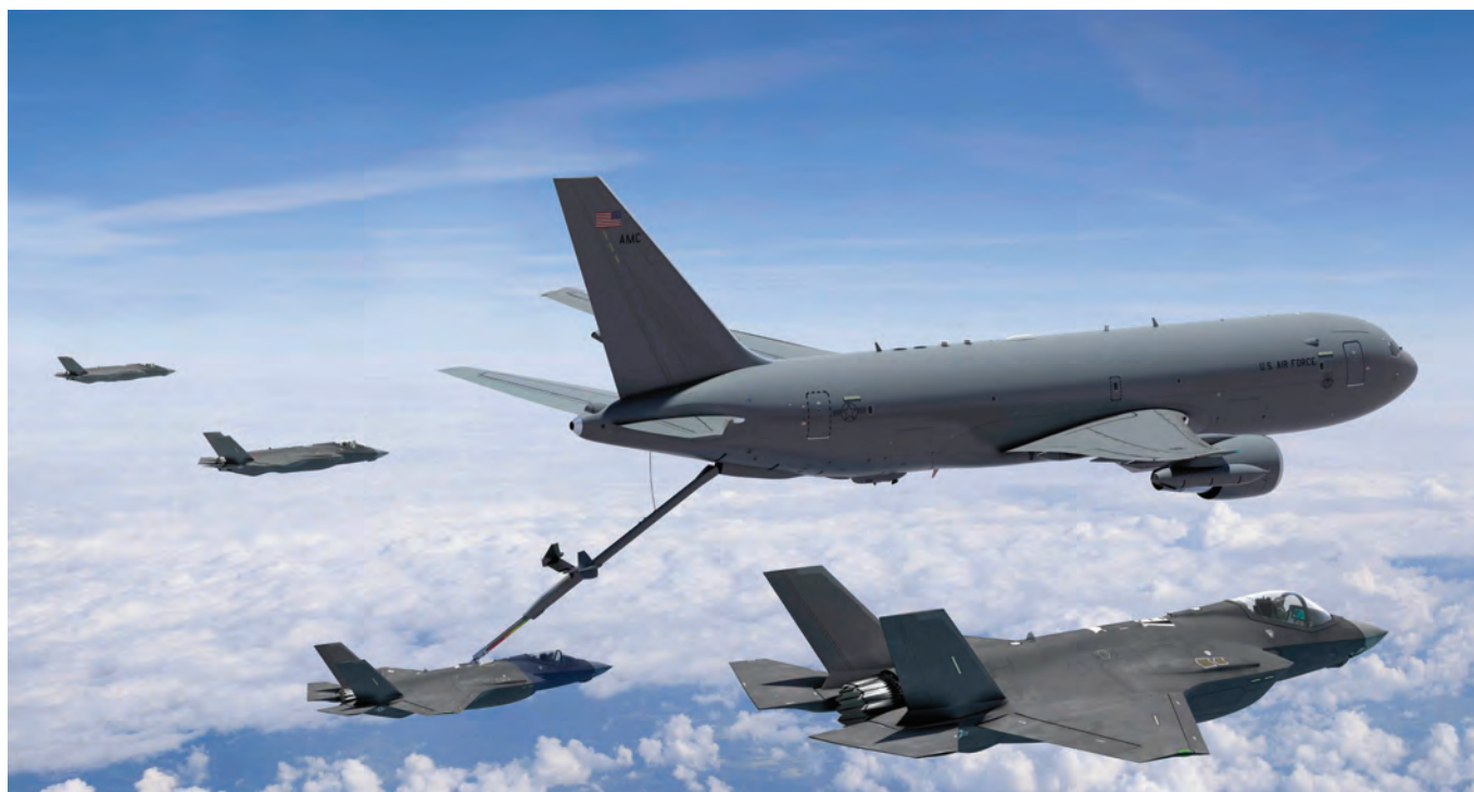
Unique among tankers, the KC-46 can operate in chemical, biological and nuclear conditions, features cockpit armor, and can operate from a large variety of smaller airfields
