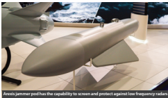
Aramis jammer pod has the capability to screen and protect against low frequency radars
