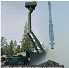
CAMM-ER has an active RF seeker that provides true all-weather performance
