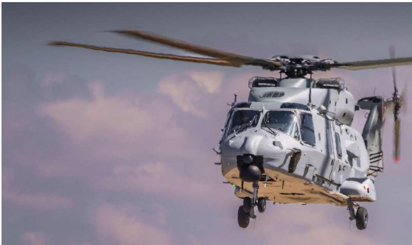
NH90 has fly-by-wire all-electric flight controls
