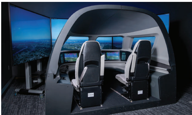
Collins Aerospace uses its experimental flight deck to develop and test semi-autonomous technology that will simplify flight
