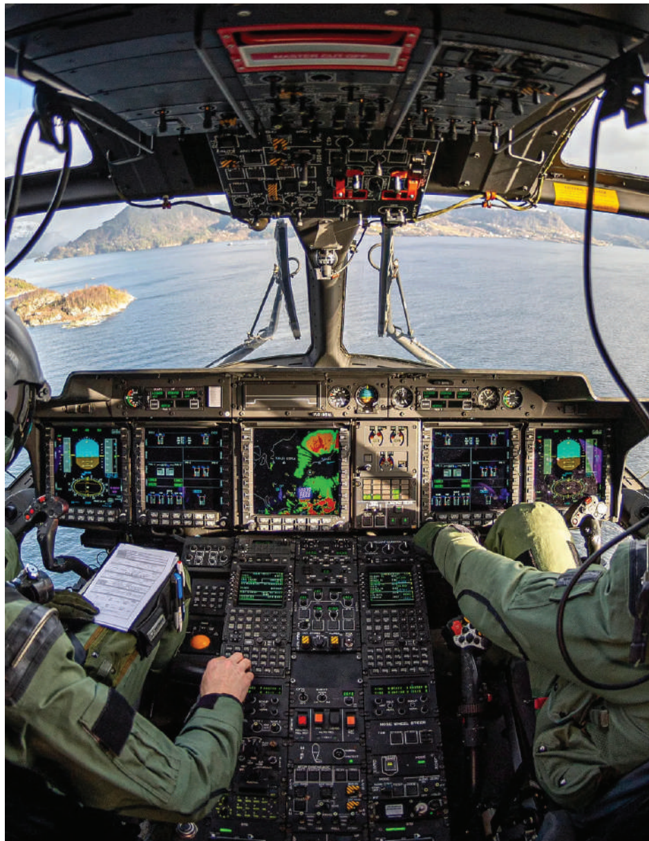
NH90's advanced avionics include precision navigation and deck landing aids
