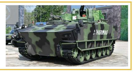
the vehicle is fitted with modular survivability kits. These include armour packages to protect against ballistic threats, mines, and improvised explosive devices (IEDs). There is also provision for an optional active protection system capable of defeating rocket-propelled grenades and anti-tank guided missiles.
