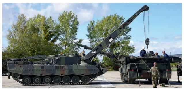
Based on the chassis of the Leopard 2 main battle tank, the Bergepanzer 3 Büffel Armoured Recovery Vehicle (ARV) has remained one of the most effective systems of its kind for over three decades.
