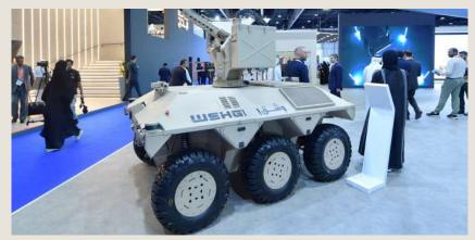
Equipped with a 6x6 all-wheel-drive system, fully independent double wishbone suspension, and differential locks on all axles, WSHG delivers unmatched off-road performance. The platform's switchable two and four-wheel steering enhances stability at high speeds and facilitates tight turns at low speeds, providing operational flexibility across various terrains.
